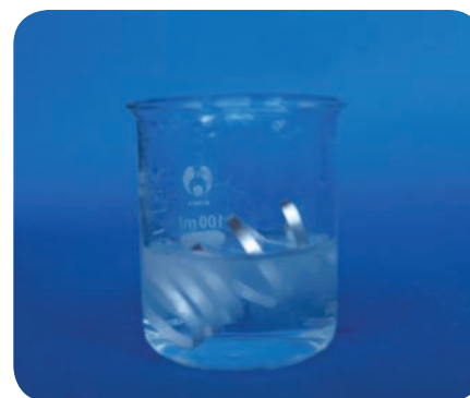
▲ Magnesium displacing hydrogen from hydrochloric acid.
