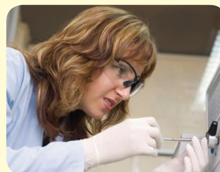
▲ Injecting a sample into the carrier gas, at the start of gas chromatography.
