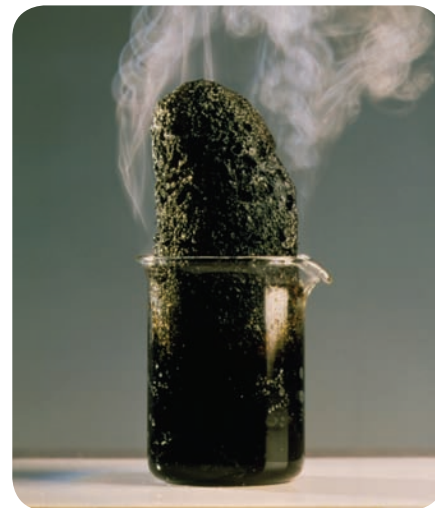
▲ Concentrated sulfuric acid was added to two teaspoons of sugar – and this is the result. It turned the sugar into carbon. Think what it could do to flesh!
